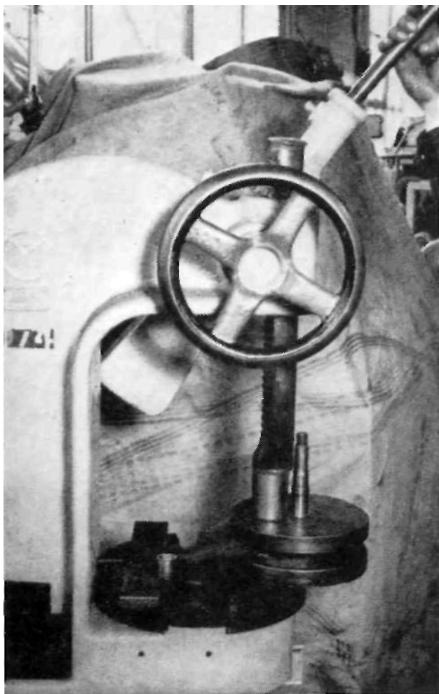
FIG. 27 Arbour Press for Flywheels
